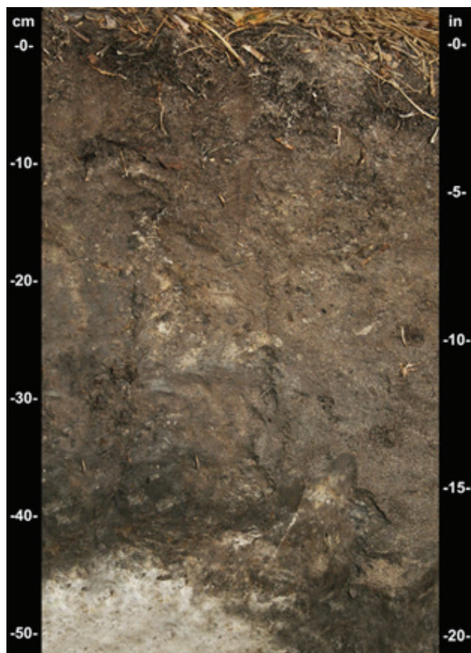
Figure 32.—Indicators F6, Redox Dark Surface, and F7, Depleted Dark Surface. A soil that meets the requirements of indicator F7 commonly also meets the requirements of indicator F6. If the dark surface layer has depletions, it most likely also has concentrations.
