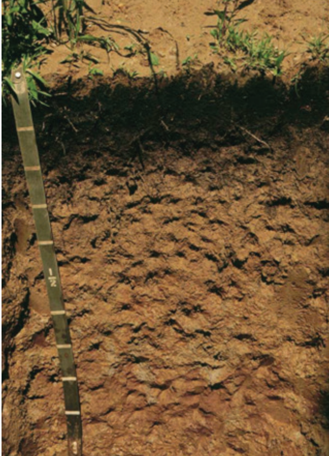
Figure 40.—Indicator F20, Anomalous Bright Loamy Soils. This indicator is restricted to areas near estuarine marshes or water. It does not require a matrix color with chroma of 2 or less.
