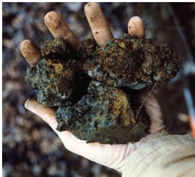
Figure 50.— Glaucconitic soils typically have gleyed, green, or black matrices and can have mottles of weathered sulfides that can be mistaken for redox concentrations. If the weathered sulfides in this glauconitic soil were mistaken for redox concentrations, this nonhydric soil would appear to meet the requirements of indicator F6, Redox Dark Surface.
