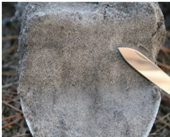
Figure 25.—Indicator S6, Stripped Matrix. This indicator requires diffuse splotchy patterns with rounded areas stripped of organic matter or iron as exemplified in this photo of a horizontal cross-section of a profile.
