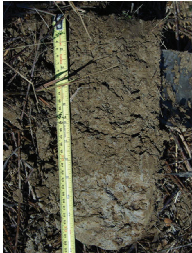
Figure 4.—The lower portion of this soil profile meets the color and depth requirements of indicator F3, Depleted Matrix; however, the upper portion of the profile contains a layer with chroma of 2 or more that is more than 15 cm (6 inches) thick. As a result, the requirements of indicator F3, Depleted Matrix, are not met.
