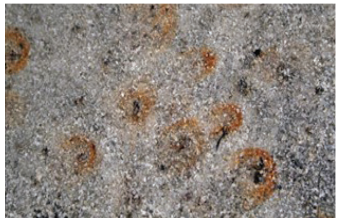
Figure 24.—Indicator S5, Sandy Redox. A close-up of the layer in figure 23 that has chroma of 2 or less and at least 2 percent redox concentrations.
