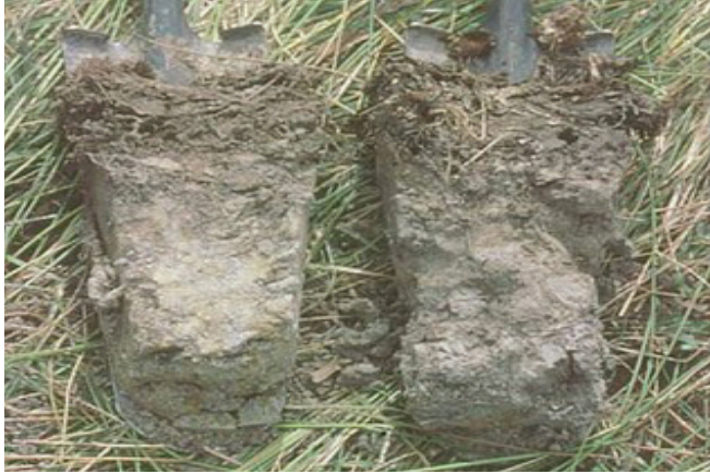
Figure 44. —The profile on the right is from a drained wetland adjacent to a ditch. The profile on the left is from an area not affected by the ditch. Both soils meet the requirements for indicators F3, Depleted Matrix, and A11, Depleted Below Dark Surface, and thus are hydric soils.
