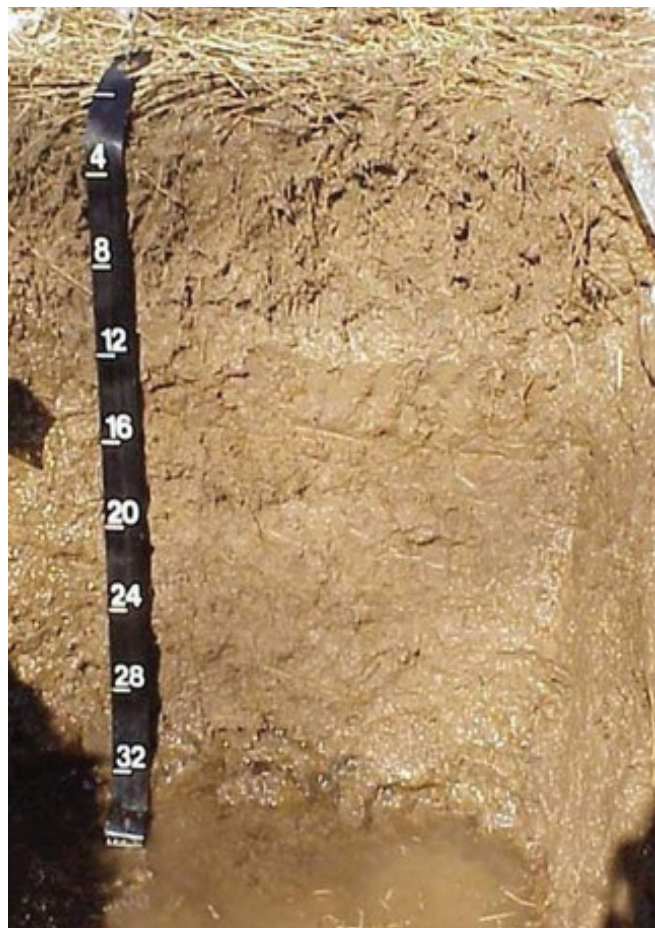
Figure 42.—Indicator F3, Depleted Matrix, in red parent material. If a soil that formed in red parent material stays wet and anaerobic long enough, it may develop the indicator F3.
