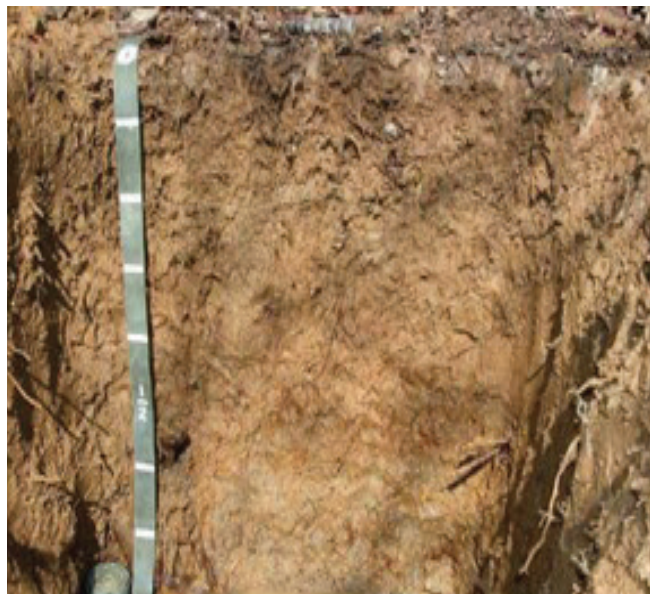
Figure 39.—Indicator F19, Piedmont Flood Plain Soils. This indicator is restricted to active flood plains. It does not require a matrix color with chroma of 2 or less.
